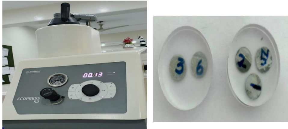
Figure 3. 5 (a) ECOPRESS for sample mounting, (b) Mounted samples
