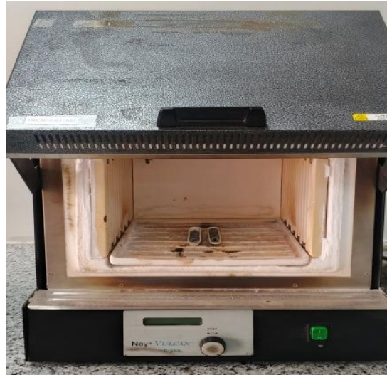
Figure 3. 2 Vulcan furnace with green pellets
