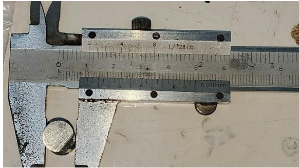
Figure 3. 4 Measuring dimensions using Vernier Caliper
