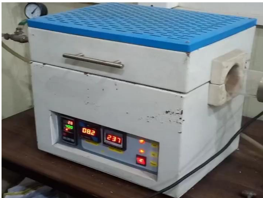
Figure 3.7 Carbonization of Coconut Shell and Pith carried out at 400 C
