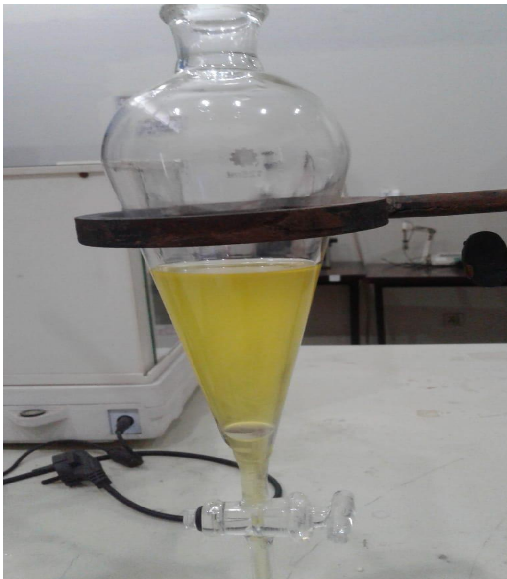
Figure 3.9 Separating Funnel Separation of Optimized Biodiesel Yielding 92%
