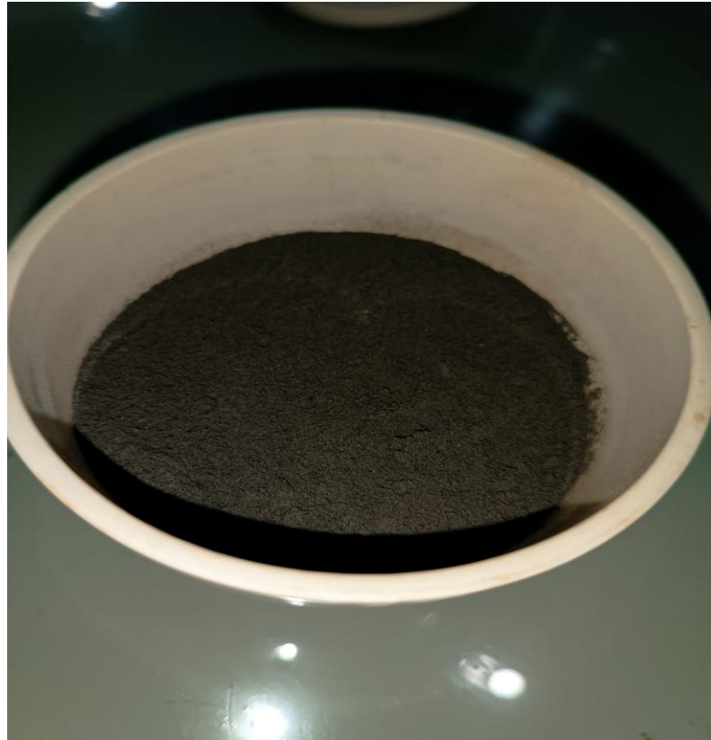
Figure 3.1 Calcined Eggshells at 600 °C after Sieve Analysis
