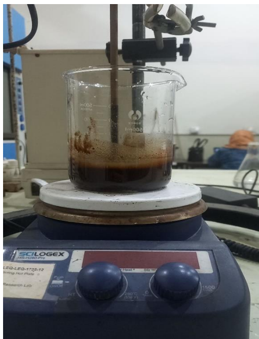
Figure 3.5 Mechanical Pre-treatment of C-CCS with 5M KOH
