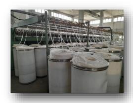
have thin wires that separate and smooth the fibers. This produces a thin cotton fabric called card sliver. At this stage, multiple card slivers are combined and stretched through a set of rollers to further align the fibers. This process helps improve the uniformity and strength of the yarn.
