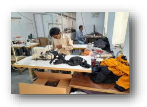
type and design requirements, different sewing techniques and stitches are used, such as straight stitch or zigzag stitch. Seam finishing techniques such as overlock binding and French seams are used to prevent fraying and improve seam durability and appearance. Clothes are adjusted many times during the sewing process to achieve the desired size and shape. Adjustments may be necessary to suit
