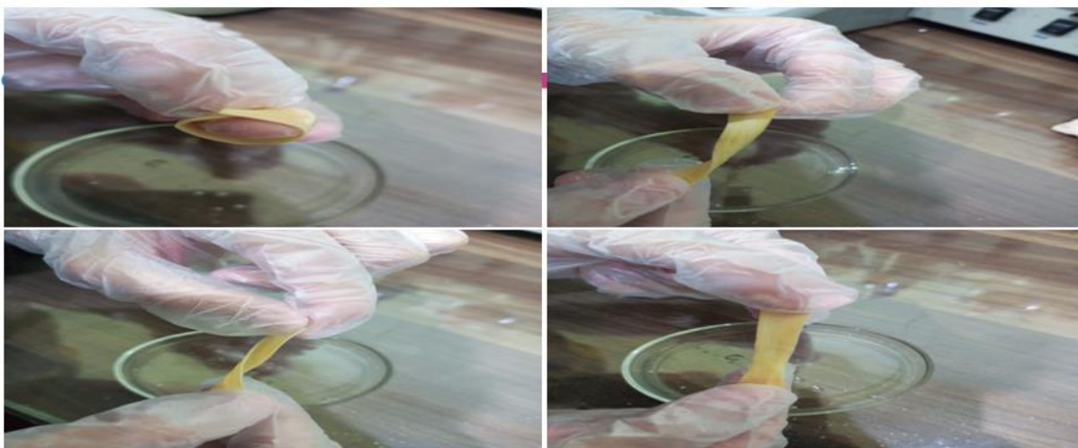
Fig. 2.5 (b) Practical demonstration of mechanical strength and flexibility for Flexible Wood. It shows that the flexible balsa wood can be totally recovered after bending.
