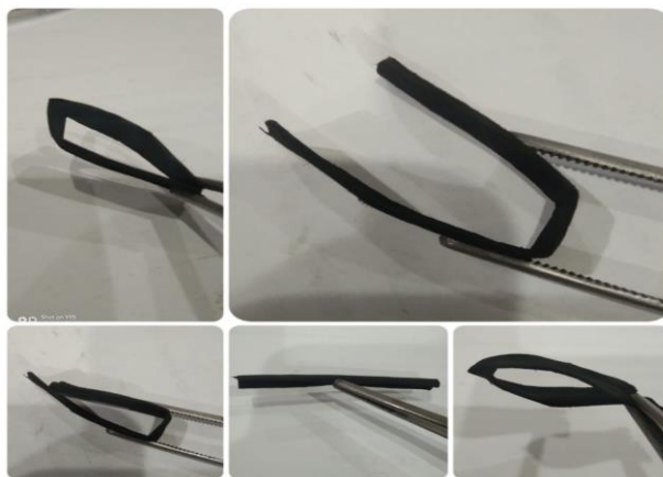
Fig 3.5 Flexibility of Balsa wood after polymerization is retained
