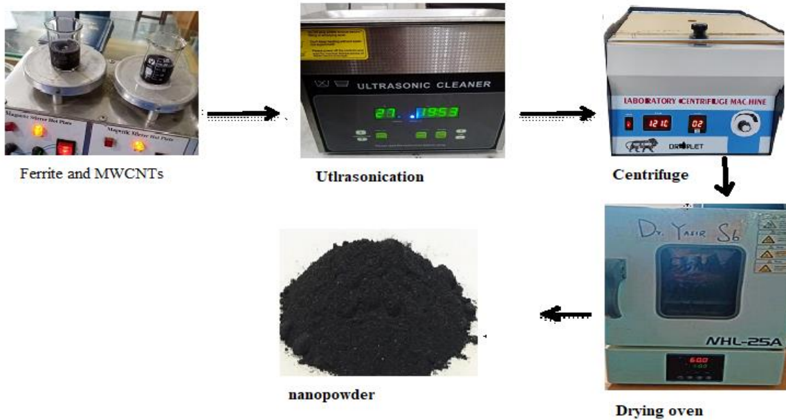
Fig 3.2: Schematic representation of CNTs deposition
