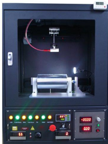
Figure 3.1 Electro-spinning & Spray unit (China), model number TL-01
