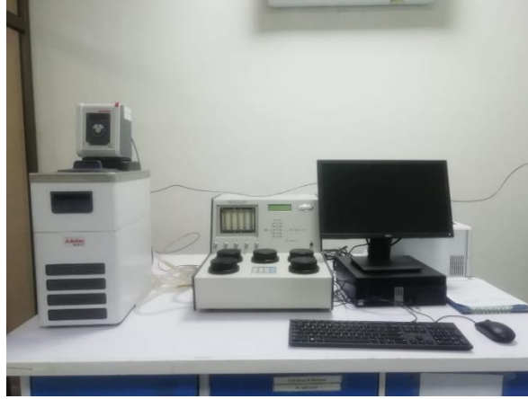
Figure 3.7 Pycnometer (PENTAPYC 5200e Automatic Density Analyzer) for density measurements
