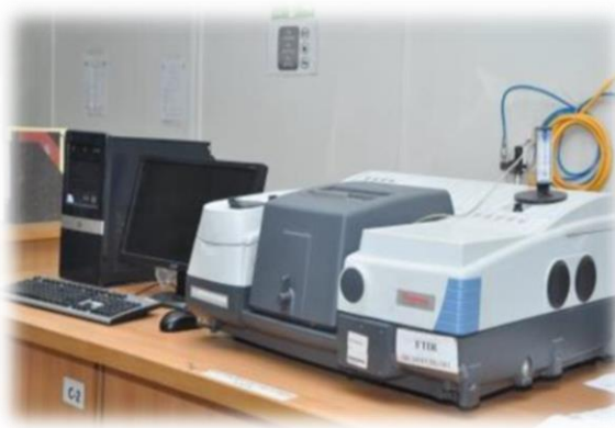
Figure 3.4 A Thermo Nicolet Scientific 6700 FTIR, USA instrument for evaluation of functional groups
