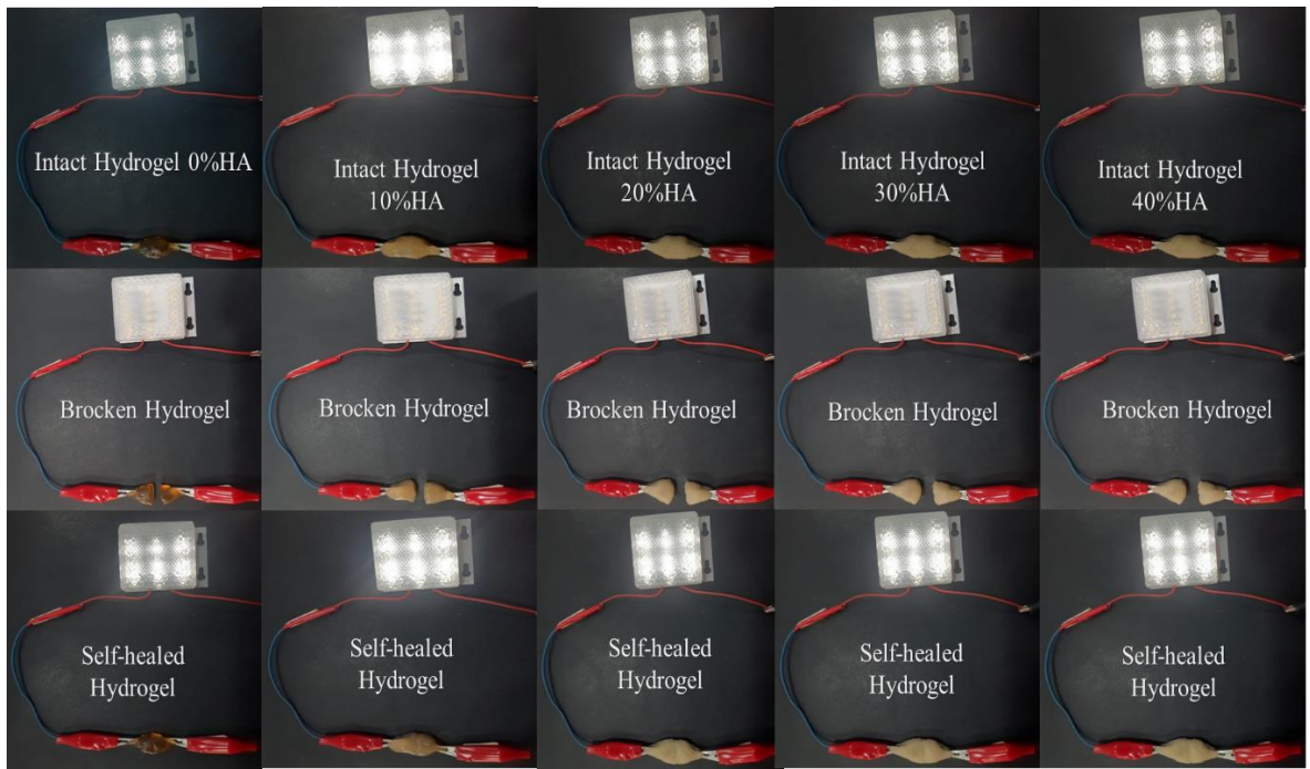
Figure 4-8 Conductivity of hydrogel
