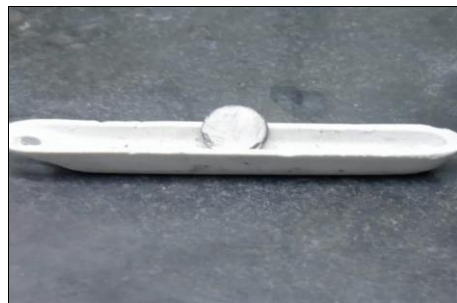
Figure 3.3: Cell (pellet) with silver paste
