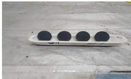
Figure 3.2: Cell (pellet) without silver paste
