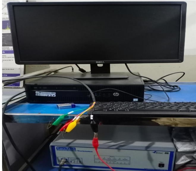
Figure 3.8 EIS measurement setup
