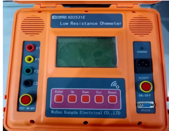
Figure 3.9 KD2531E low resistance ohmmeter for DC conductivity measurements
